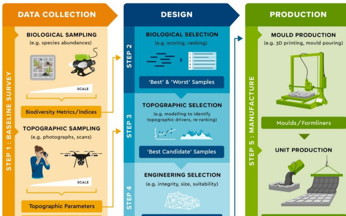
Figure 1 - Five-step process for designing natural topography-based eco-engineering interventions for marine artificial structures. Source: Evans et al. (2021)
